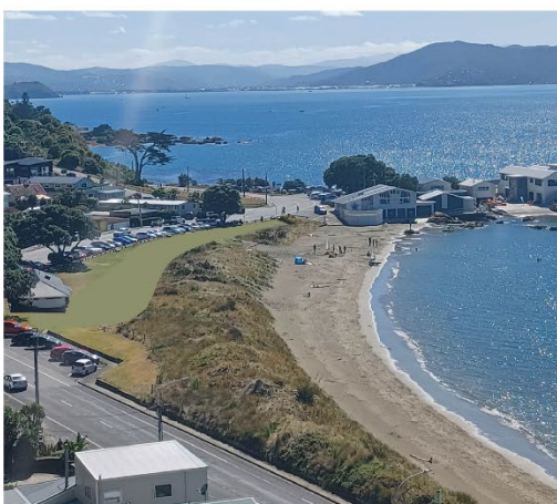
Grass reinstatement and extent of dune shifted to north end of beach
